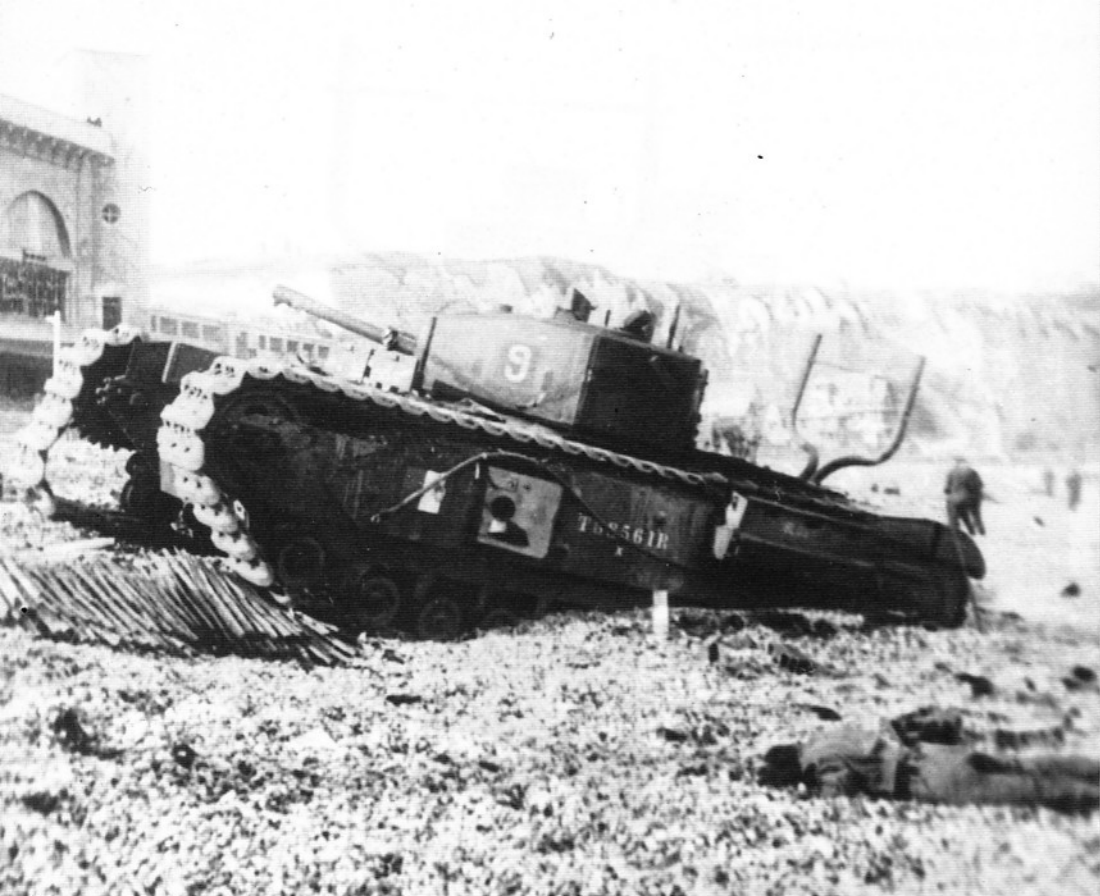
Churchill Mk. III tank of Canadian 14th Tk.Rgt. abandoned by amputate of track.
